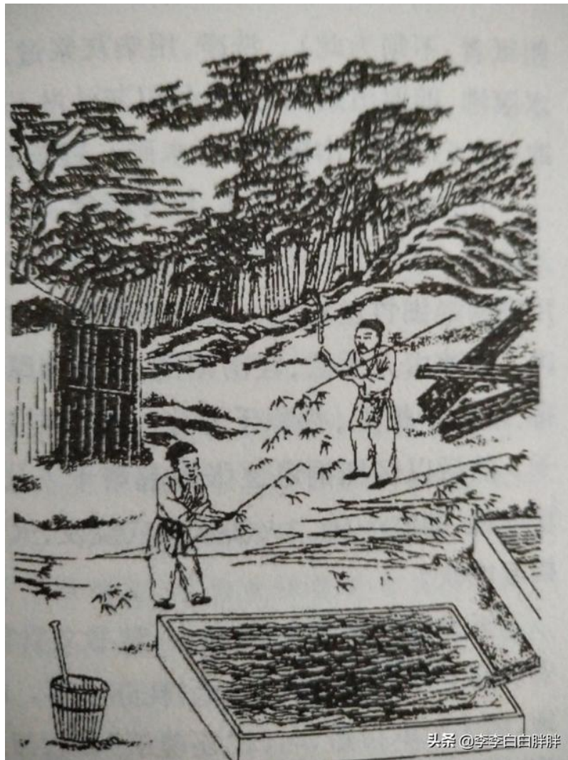
Cut bamboo is washed and steeped in a water pit to prepare material for making paper
